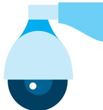
**Pan-tilt-zoom (PTZ) cameras** can typically be controlled by remote operators, programmed to scan an area with preset movements, and/or programmed to move in response to triggering events (e.g., gunshots). They typically have viewsheds of 35 degrees and use optical zooming, though they can also include digital zooming at their maximum optical zoom settings.
