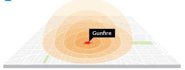
Acoustic sensors throughout the city listen for the distinctive waveforms that firearms produce. When detected, individual sensors calculate the distance to the sound.
